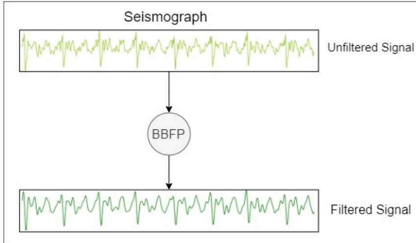
Figure 2.3: *Signal Filtering Using a 5<sup>th</sup> Order Butterworth Band-pass Filter*
