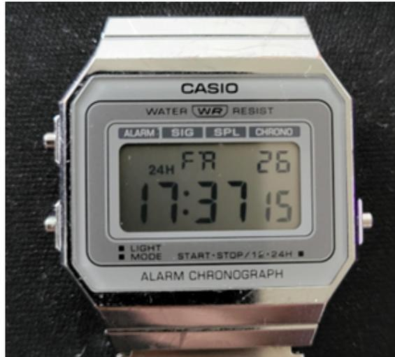
Figure 3.1: Timekeeping Mode of the digital watch. The mode button is the under-left button. The light button is the upper-left button. And the right button is for changing the time format.
