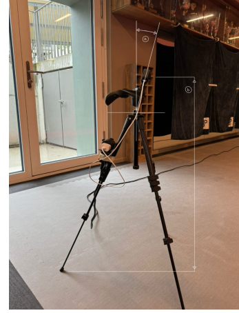
Figure 3.2: The camera is set up exactly one meter from the tatami corner away on the diagonal. Denoted by a is the angle between camera and the middle axis, and by b the distance from the ground to the camera lens exactly one meter up from the ground.
